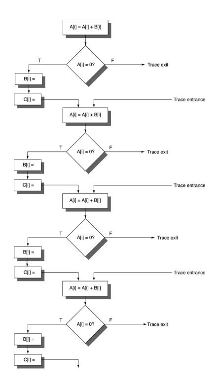
This trace is obtained by assuming that the program fragment in Figure 4.8 is the inner loop and unwinding it four times, treating the shaded portion in Figure 4.8 as the likely path.
